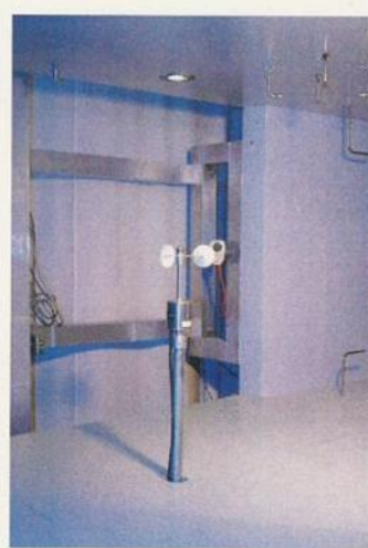
Calibration set-up of the anemometer calibration in the wind tunnel of Deutsche WindGuard, Varel. The anemometer shown is of the same type as the calibrated one. Remark: The proportion of the set-up are not true to scale due to imaging geometry.
