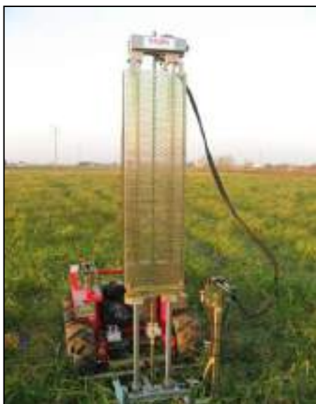
Fig.11: Penetrometro dinamico continuo (DPM – PAGANI Geotechnical Equipment)
