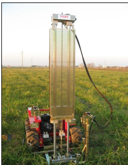
Fig.12: Penetrometro dinamico continuo (DPM – PAGANI Geotechnical Equipment)
