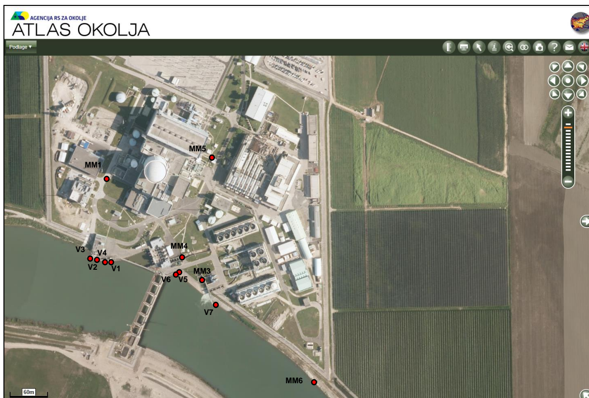
Figure 6: Locations of discharges and measuring points of NEK waste water
