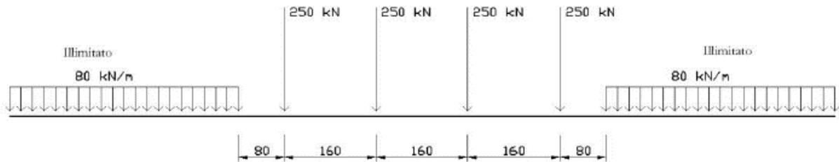
$$Q_{vk} = 250 \text{ kN} \quad q_{vk} = 80 \text{ kN/m}$$
