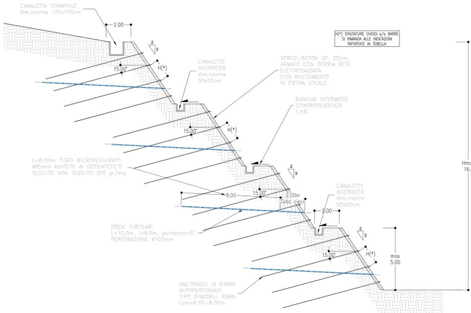
**SOIL NAILING - PARTICOLARE CHIODATURA** scala 1:10
