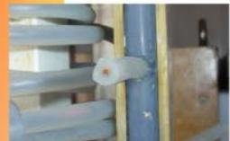
Electrode tip after three years of operation
