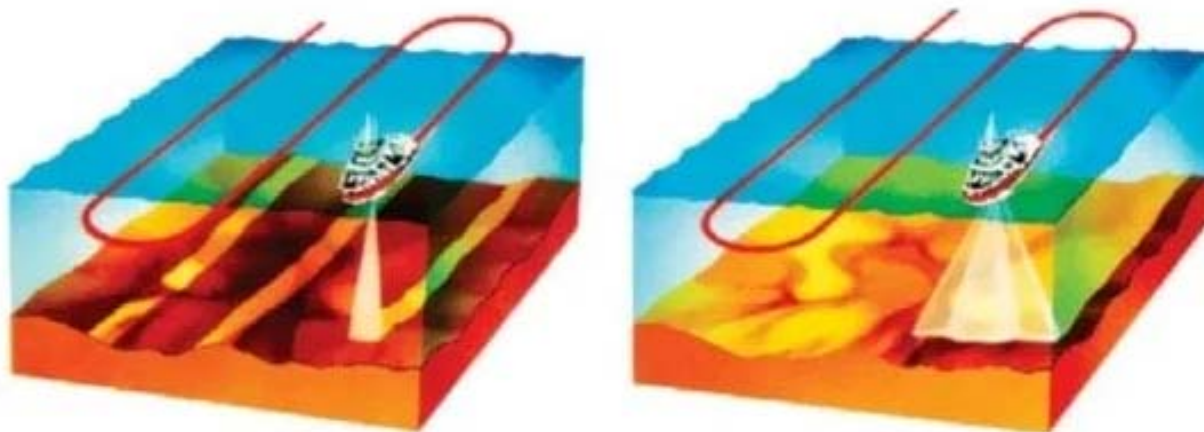
Figura 3: single beam Vs multi beam
