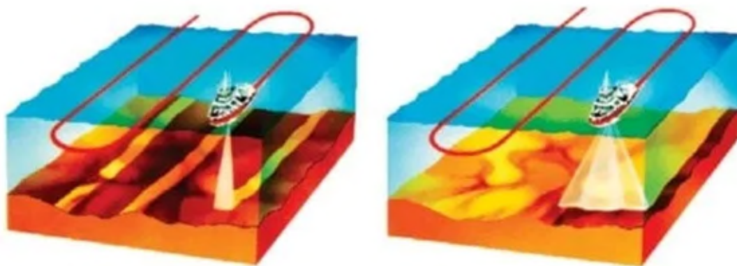
Figura 22: single beam Vs multi beam
