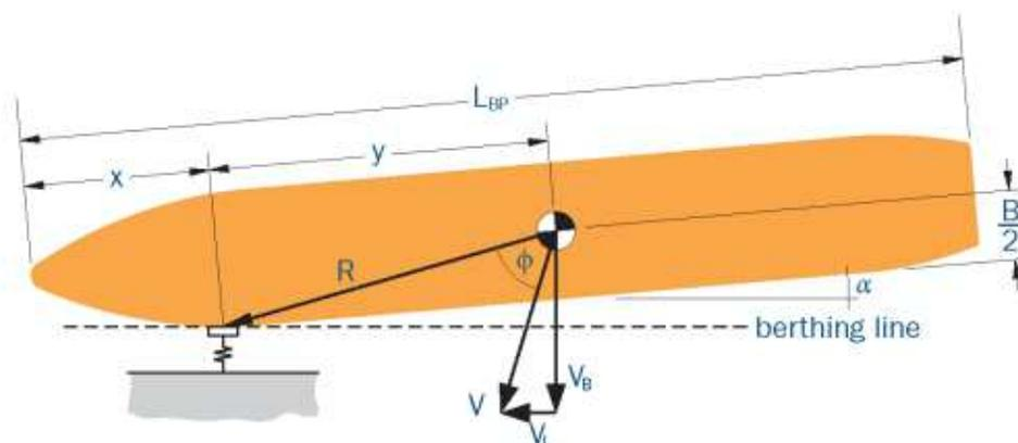
$V_L$  = longitudinal velocity component (forward or astern)
