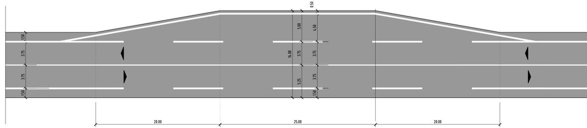
SCHEMA PLANIMETRICO TIPO "C1" (D.M.05/11/01)
