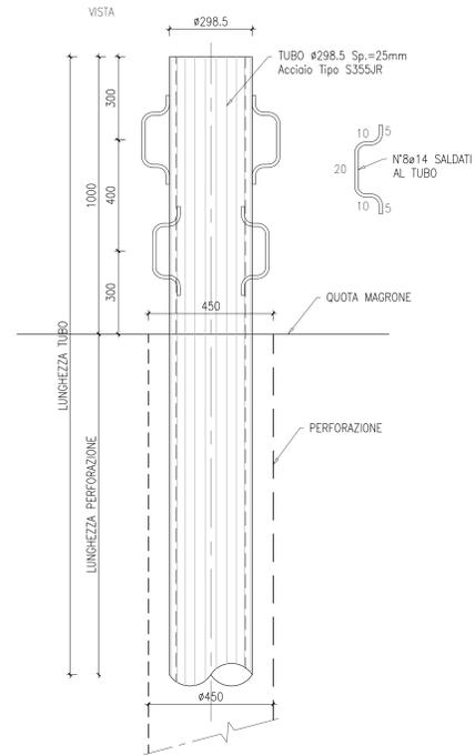
CARATTERISTICHE MEDIOPALO SPALLA (Rotary)
