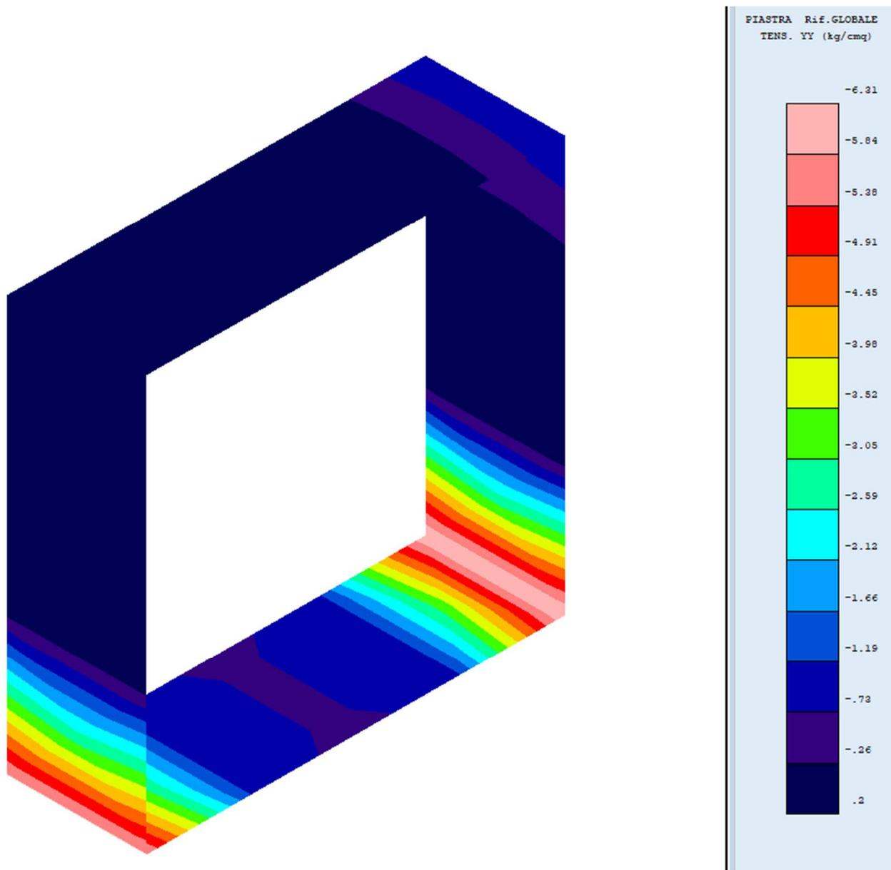
Figura 12: Tensore yy – SLE quasi perm. comb. 1
