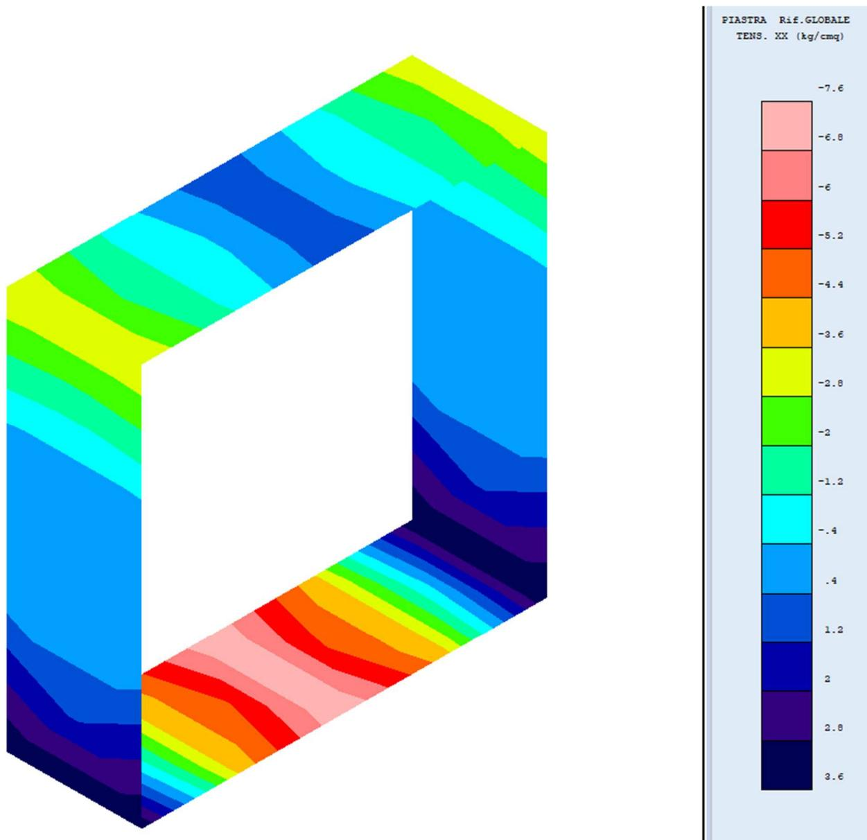
Figura 11: Tensore xx – SLE quasi perm. comb. 1
