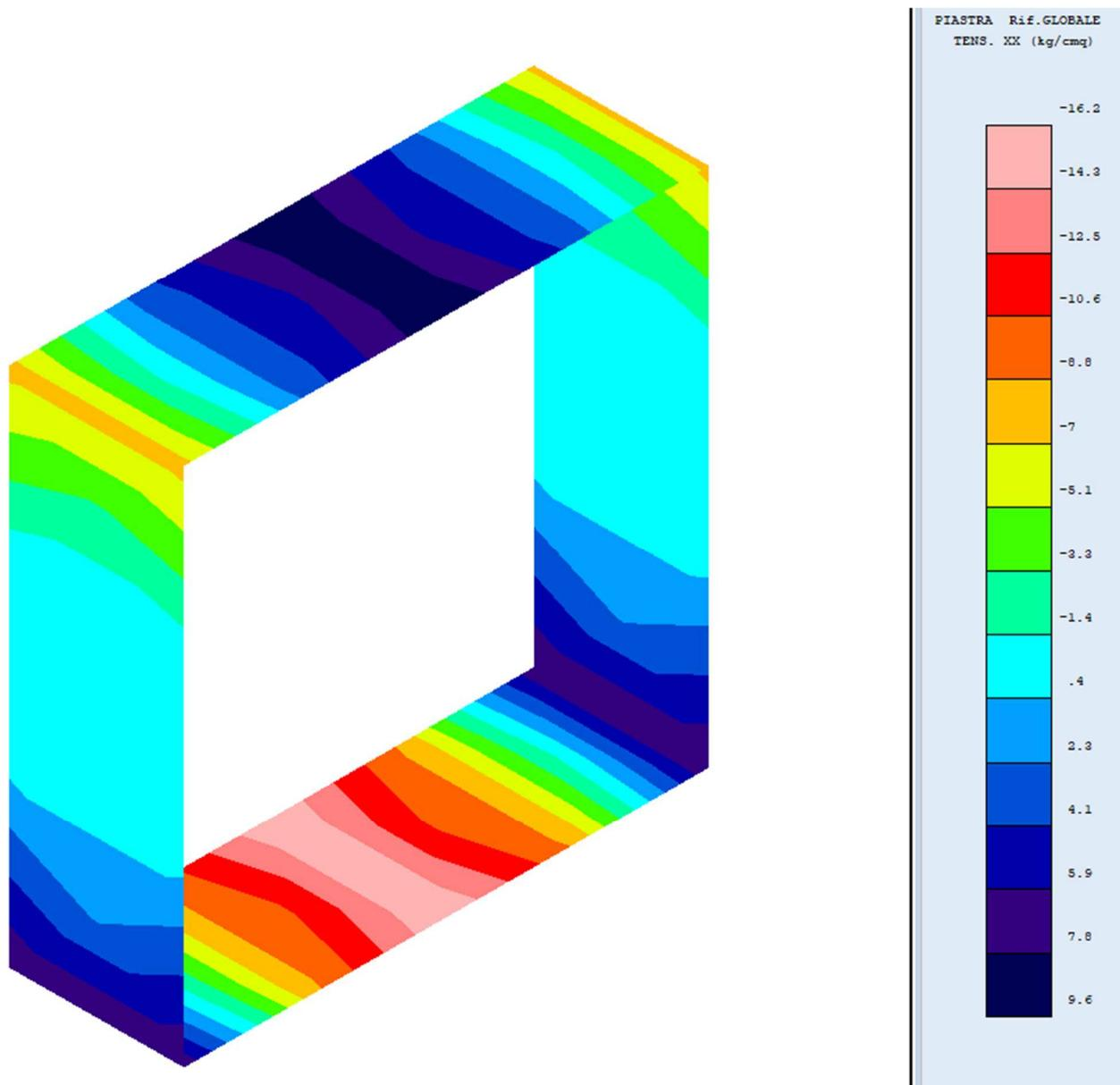
Figura 9: Tensore xx – SLE freq. comb. 1
