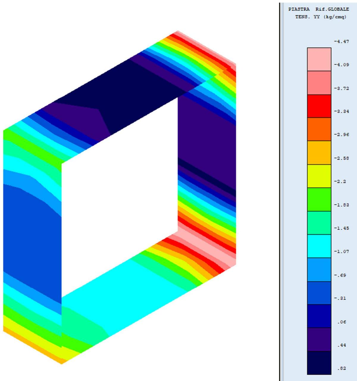
Figura 12: Tensore yy – SLE quasi perm. comb. 1
