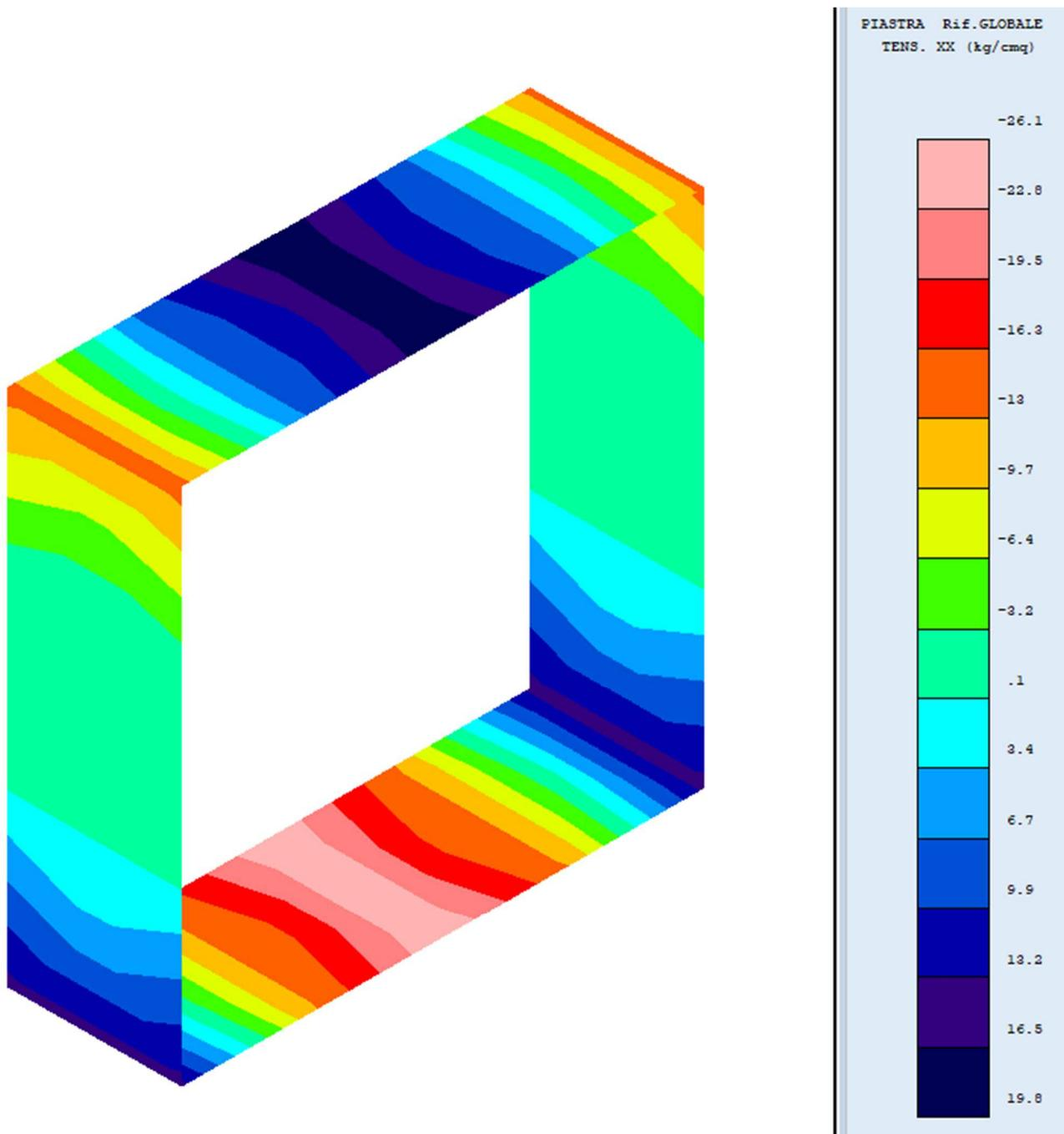
Figura 9: Tensore xx – SLE freq. comb. 1
