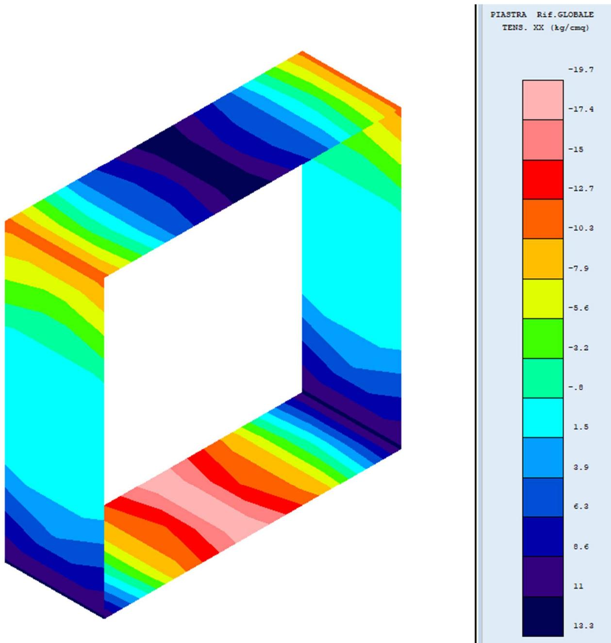
Figura 11: Tensore xx – SLE quasi perm. comb. 1
