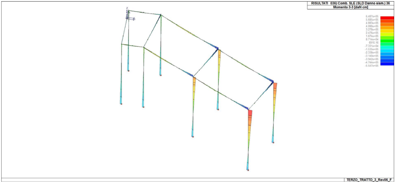
43_RIS_M3_036_Comb. SLE (SLD Danno sism.) 36
