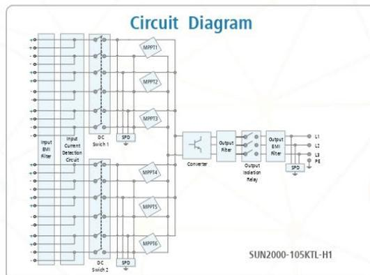
Figura 6: datasheet inverter
