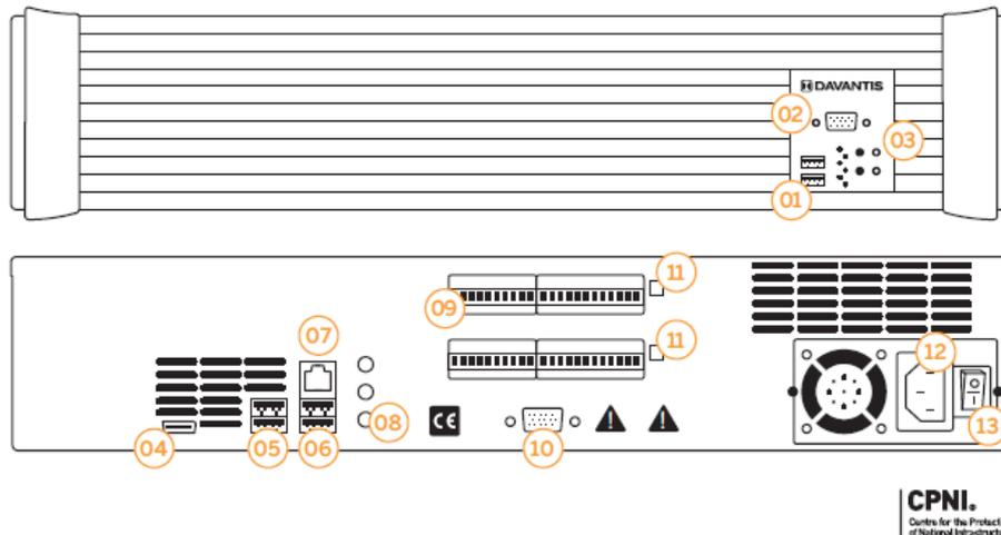
01 - 2 USB 2.0 connections 02 - 1 VGA connection 03 - 1 On/Off switch 04 - 1 HDMI connection 05 - 2 USB 3.0 connections 06 - 2 USB 2.0 connections 07 - RJ45 network connector 10/100/1000 08 - 1 audio Jack 3.5 input/output port 09 - 8 inputs N/O or N/C 10 - 1 VGA connection 11 - 4/8/12/16 internal relay outputs N/C (optional) 12 - 1 slot for power cable 13 - 1 On/Off switch for power supply
