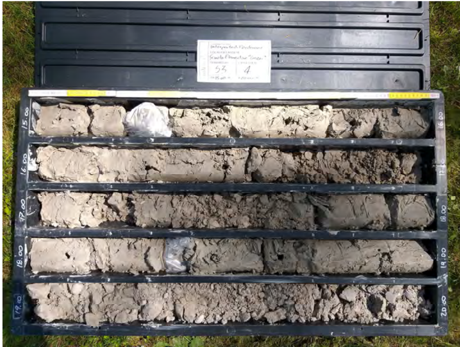
Sondaggio S3, cassetta N° 4, da 15,0 m a 20,0 m
