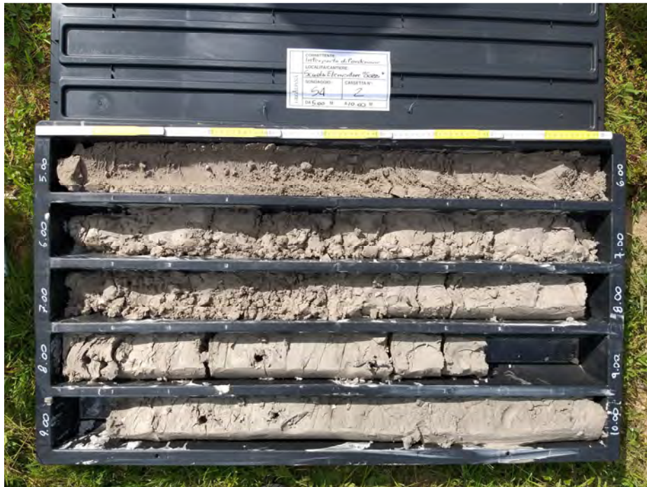
Sondaggio S4, cassetta N° 2, da 5,0 m a 10,0 m
