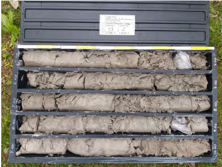
Sondaggio S3, cassetta N° 2, da 5,0 m a 10,0 m
