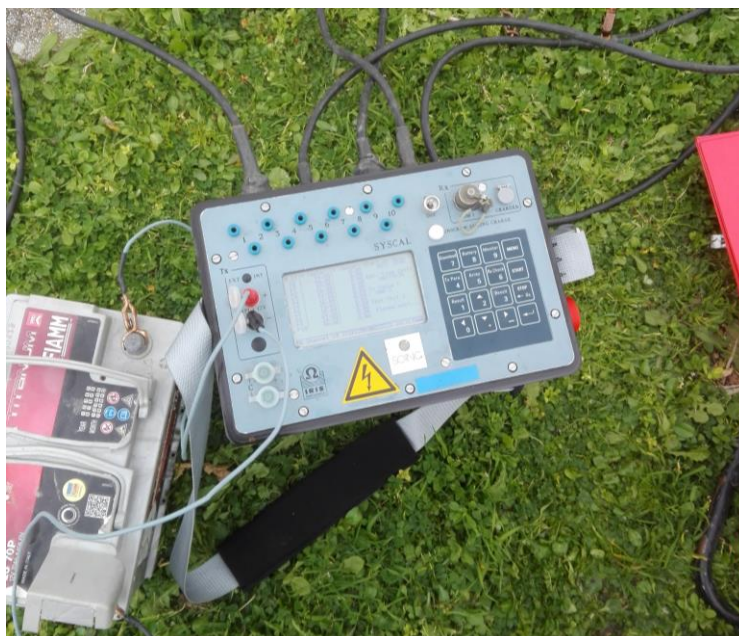
Figura 2.1.1.1: Georesistivimetro - Syscal Pro (Iris Instruments).
