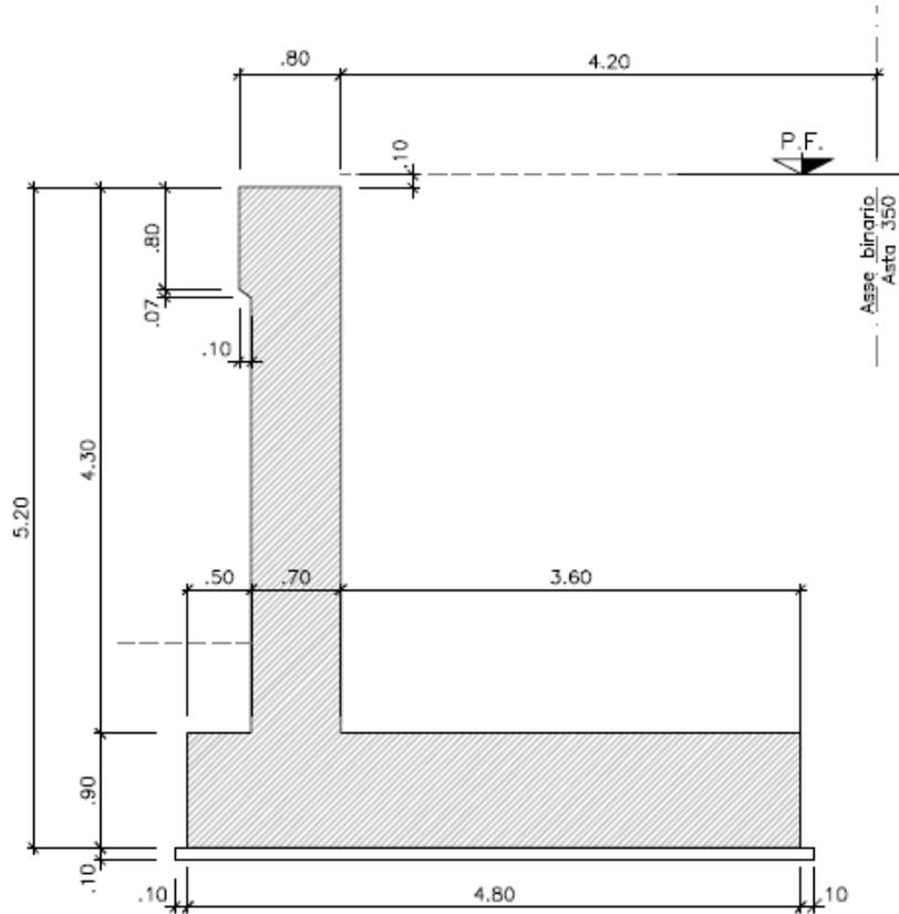
Figura 3 – Carpenteria muro MU07 TIPO B
