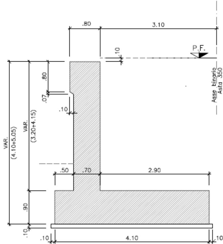
Figura 2 – Carpenteria muro MU07 TIPO A
