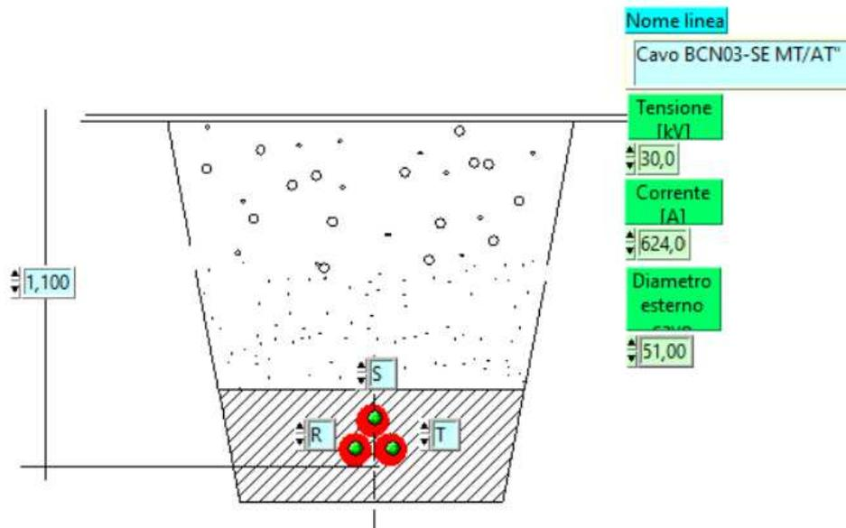
Figura 2: Posa cavo 30 kV "BCN03-SE MT/AT"
