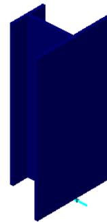
Si ottiene  $\sigma = \sqrt{(\sigma_x^2 + 3 \tau_z^2)} = 163 \text{ N/mm}^2 < 355/1.05 = 338 \text{ N/mm}^2$
