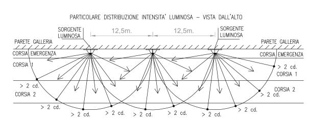
INTENSITA' LUMINOSA DELLA PLAFONIERA PLO8 SU CONO DI 15' IN CONFORMITÀ' A UNI EN 16276/13
