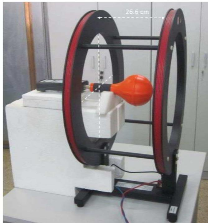
**Figure 2: Calibration set-up in the Helmholtz coils system – B field**
