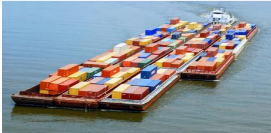
Figure 2-7 Typical river push-tow barge system
