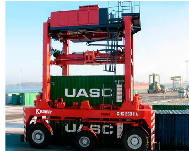
Figure 9-4 Straddle carrier, source KALMAR straddle carrier catalogue
