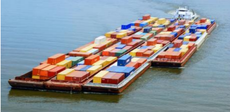
Figure 3-6 Typical river push-tow barge system
