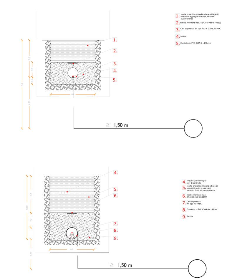
PARTICOLARE PARALLELISMO TRA CAVIDOTTI BT- MT E TUBAZIONI METALLICHE SU STRADA STERRATA O TERRENO AGRICOLO SCALA 1:10 (QUOTE IN m)
