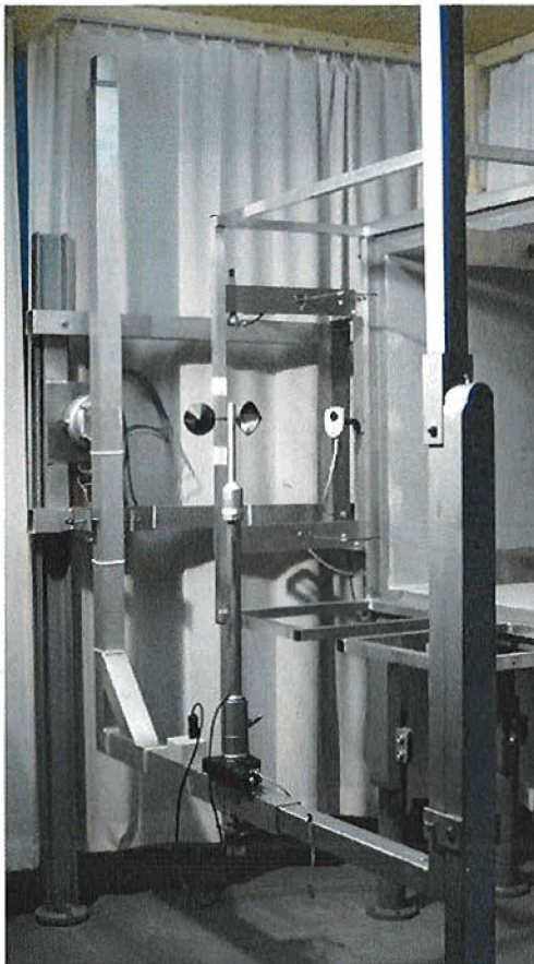
Calibration set-up of the anemometer calibration in the wind tunnel of Deutsche WindGuard, Varel.
