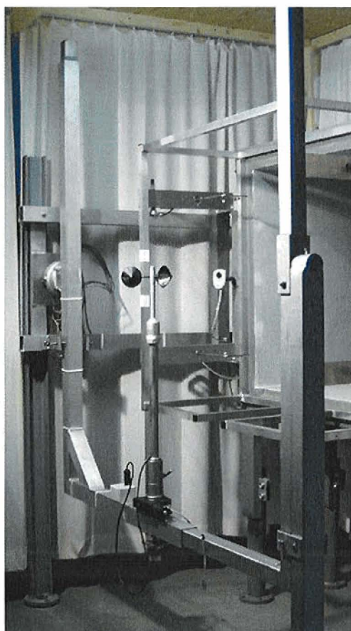
Calibration set-up of the anemometer calibration in the wind tunnel of Deutsche WindGuard, Varel. The anemometer shown is of the same type as the calibrated one. Remark: The proportion of the set-up are not true to scale due to imaging geometry.
