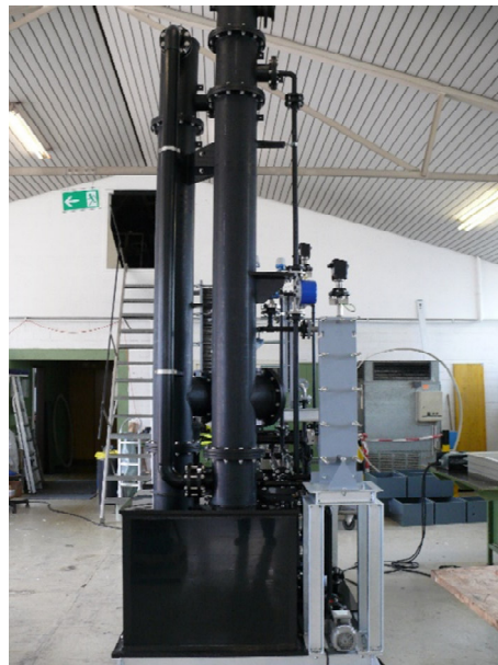
Compact gas scrubber DN150 with two scrubbing columns and heat exchanger
