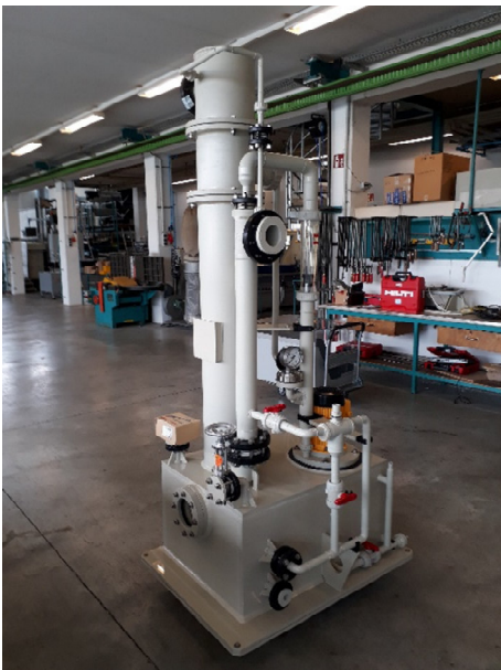
Compact gas scrubber DN80 with submerged pump
