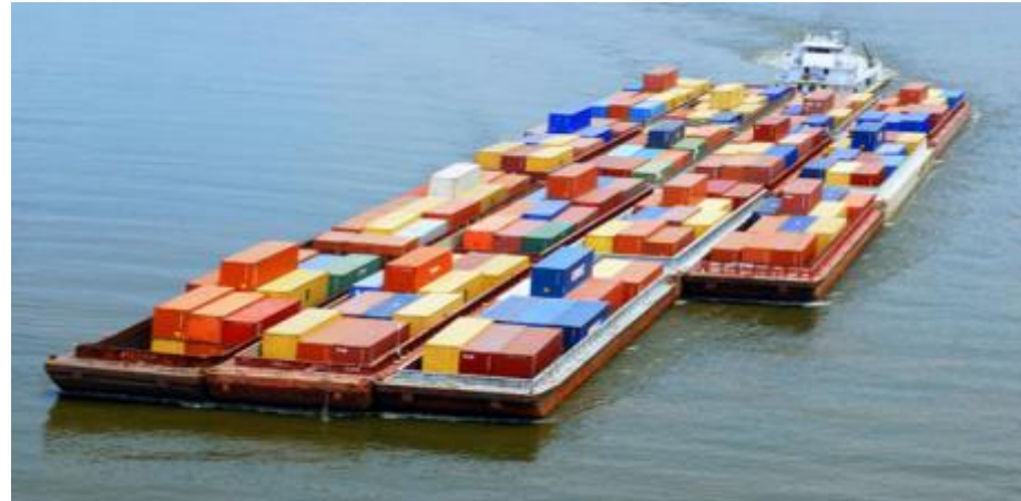
Figure 2-7 Typical river push-tow barge system
