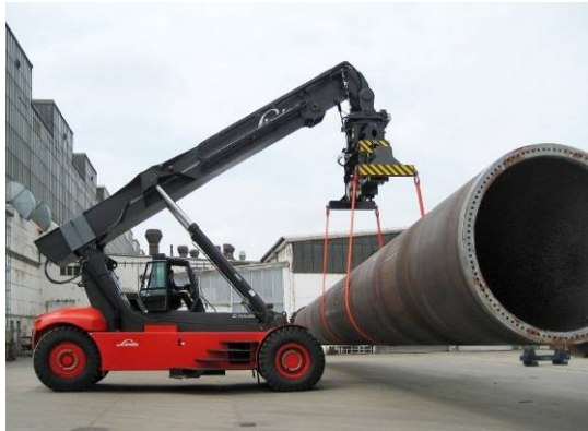
Figure 9-5 Reach stacker handling out of gauge cargo, source ConTraiLo “Linde Reach Stacker”
