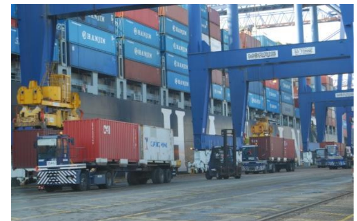
Figure 6-8 Transfer between ship to shore cranes to stack crane, here performed by tractor trailer units
