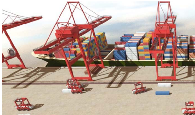
Figure 9-2 Automated shuttle carrier operation in the crane back reach, source Kalmar shuttle carrier catalogue
