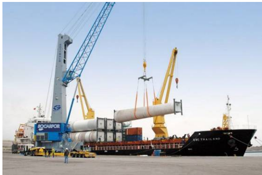
Figure 9-6 Mobile harbour crane to handle out of gauge cargo, photo shows Model 7, G HMK 7408 B four-rope crane handling wind turbine components at Socarpur, Portugal – Source http://www.setcorp.ru
