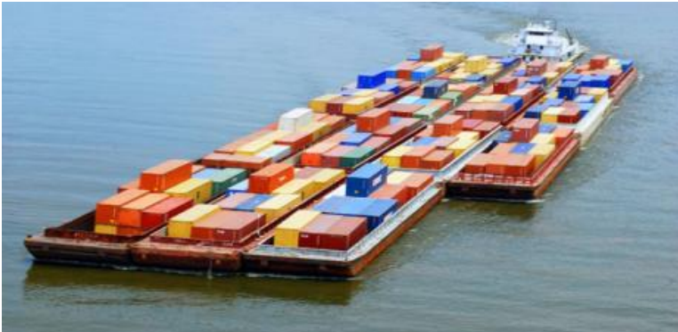
Figure 3-6 Typical river push-tow barge system
