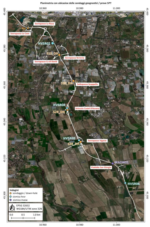
PROVE SISMICHE IN FORO DOWN-HOLE
