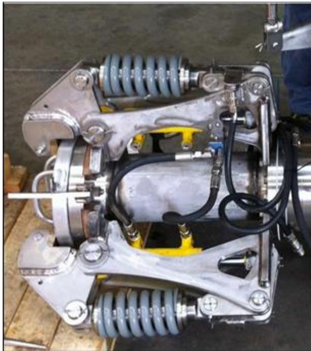
**Figura 11** - Quick Connect / Disconnect Coupler
