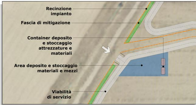
DETTAGLIO 3 AREA DI CANTIERE - SCALA 1:500
