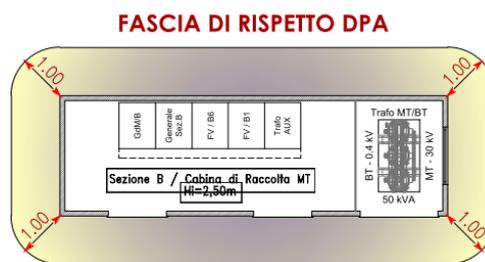
$$\begin{array}{l} \text{TRAFO 50 kVA} \longrightarrow I = 72 \text{ A} \\ \text{CAVI 1x35 mmq} \longrightarrow D_e = 14,6 \text{ mm} \end{array}$$
