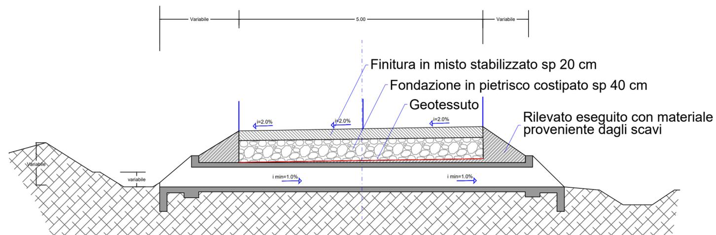
DETTAGLIO MANUFATTO IMBOCCO/SBOCCO\_SCALA 1:50
