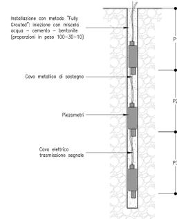
LE CELLE PIEZOMETRICHE VERRANNO INSTALLATE SECONDO IL METODO "FULLY GROUTED"; IN CIASCUN FORO VERRANNO INSERITE 3 CELLE PIEZOMETRICHE, IN CORRISPONDENZA DEI LIVELLI PIÙ INTERESSANTI PER IL MONITORAGGIO PIEZOMETRICO.
