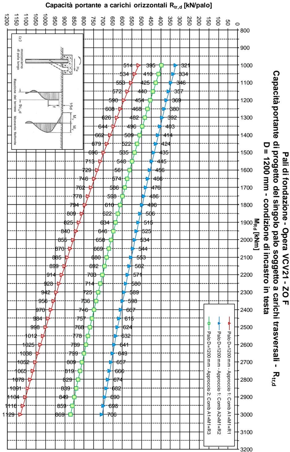
FIGURA 5-2: CAPACITÀ PORTANTE ORIZZONTALE – PALI TRIVELLATI  $\phi$  1200
