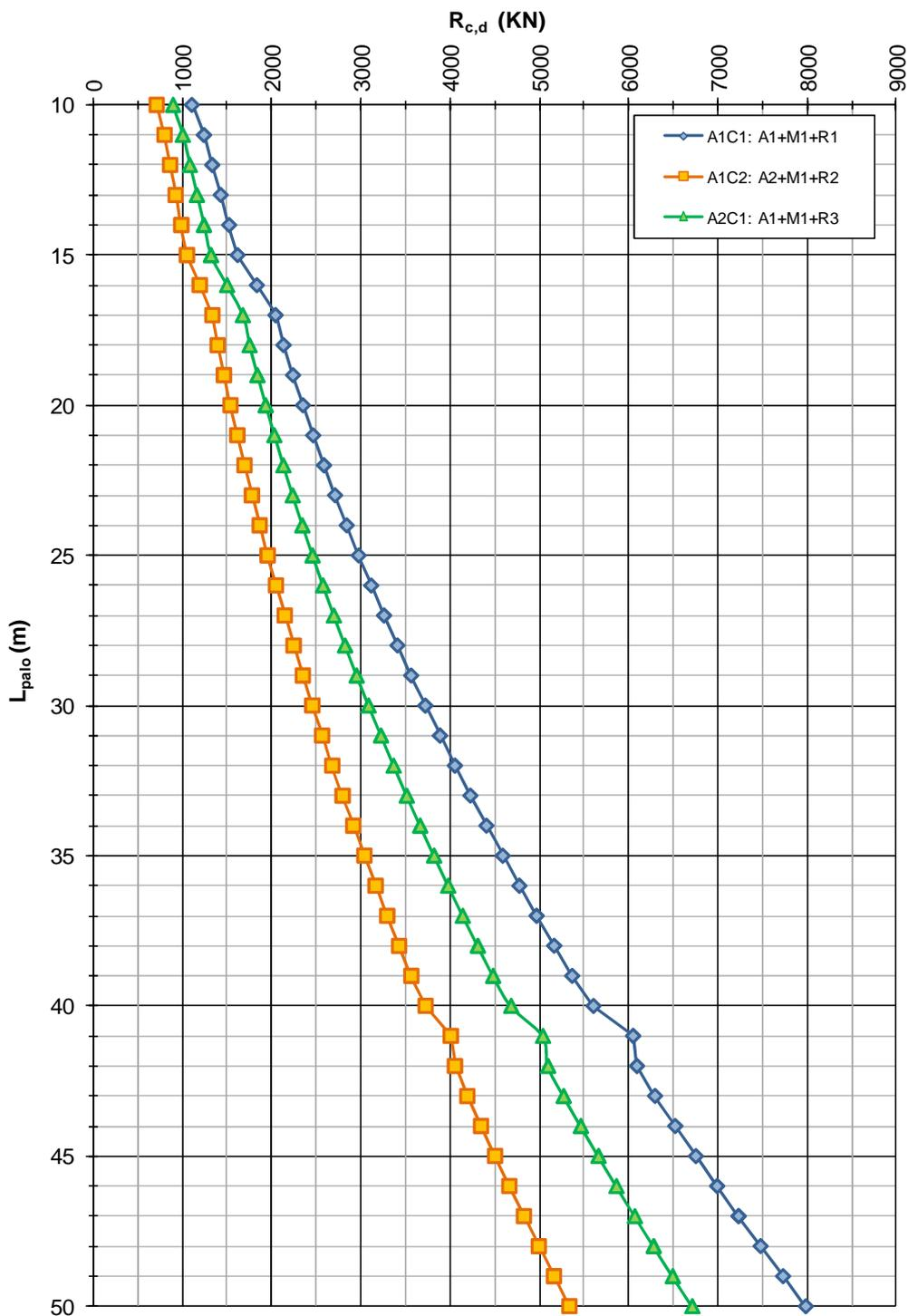
FIGURA 4-3: CAPACITÀ PORTANTE A COMPRESSIONE – PALI TRIVELLATI  $\phi$  1200
