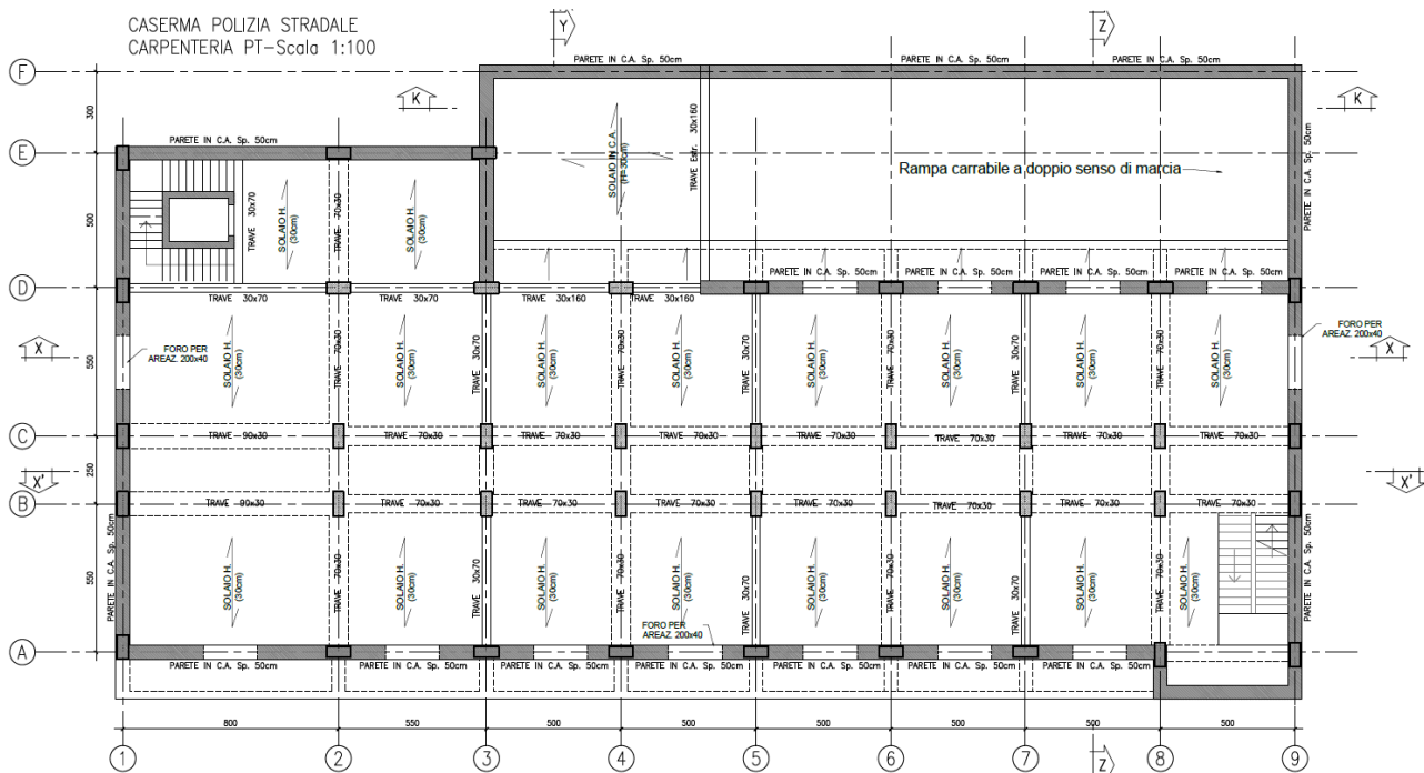
Figura 4 – Carpenteria piano terra
