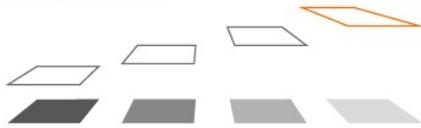
Bifacial performance is increased by height of installation, reducing shadow intensity projection.
