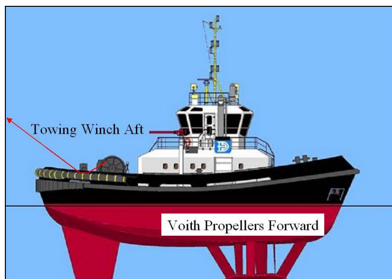
Figure 6.3 – Voith Schneider Tug in Profile
