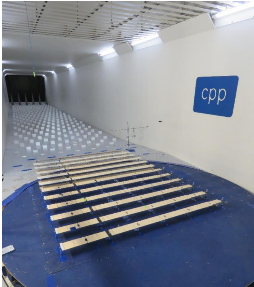
Figure 318. Wind tunnel model (array section)
