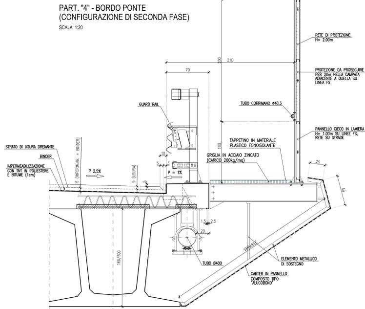
DETTAGLIO DISPOSITIVO DI RACCOLTA
