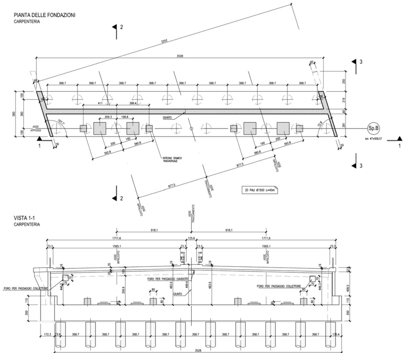
FIGURA 3-7: CARPENTERIA SPALLA B.
