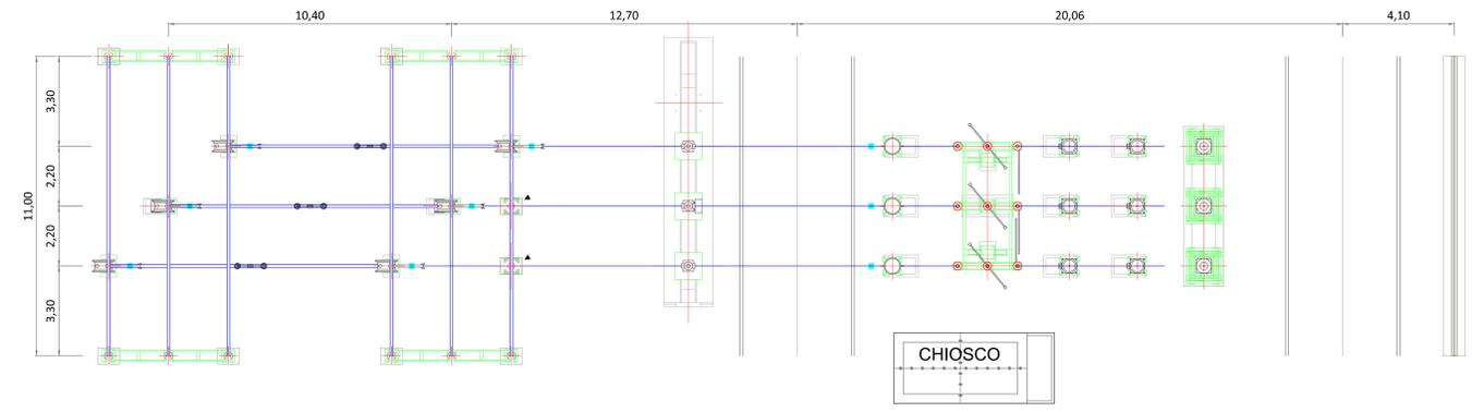
PIANTA STALLO ARRIVO CAVO PRODUTTORE 150 kV - SCALA 1:100
