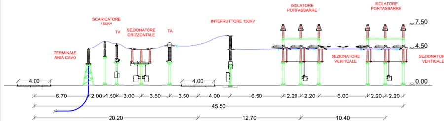
**SEZIONE D-D - PARALLELO MODELLO TRAVERSO**
