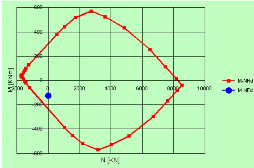
FIGURA 24 DOMINIO RESISTENTE SEZIONE TRASVERSALE ATTACCO DELLO SBALZO
