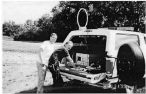
Fig. 1. Vehicle with spectrum analyzer, active loop antenna, and printer.
