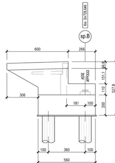
**FIGURA 3-7: CARPENTERIA SPALLE.**
