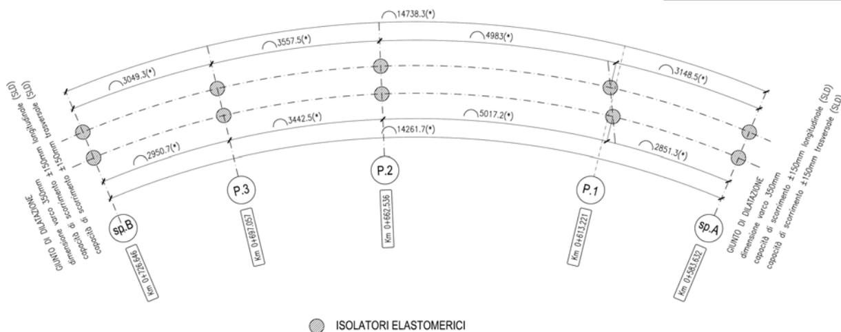
FIGURA 3-4: SCHEMA DEGLI ISOLATORI SISMICI ELASTOMERICI.
