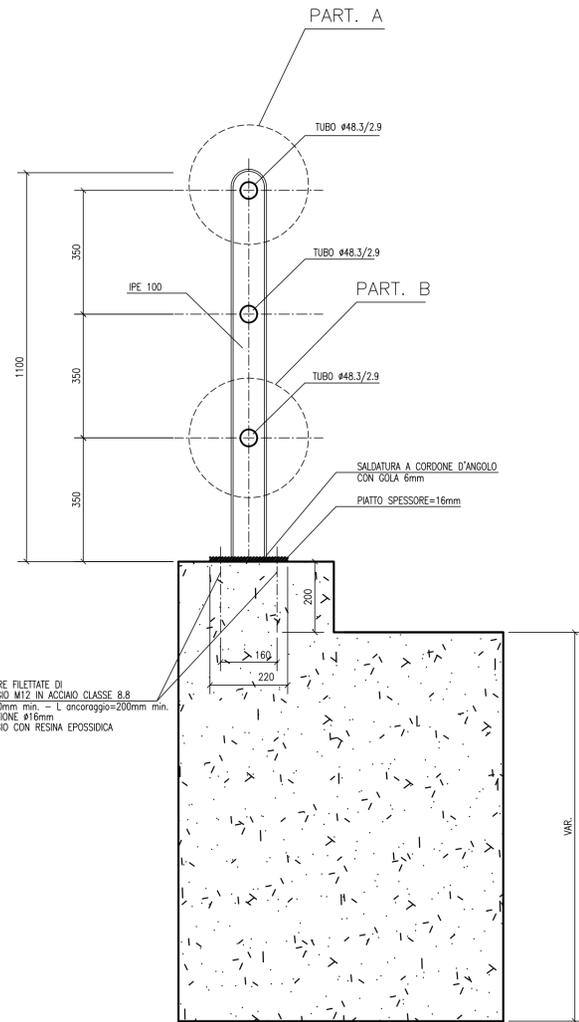
2+2 BARRE FILETTATE DI ANCORAGGIO M12 IN ACCIAIO CLASSE 8.8
